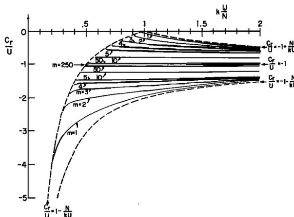
Fig. 3. Graph of  $c_r$  versus  $k$  for neutral modes in the presence of a lower boundary. Each curve is labeled by its mode number. Also shown are the boundaries of region C discussed in section 2. Note that all neutral solutions are now in region C rather than region A.
