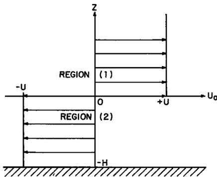
Fig. 1. Helmholtz velocity profile. For calculations in section 2 the lower boundary is removed.
