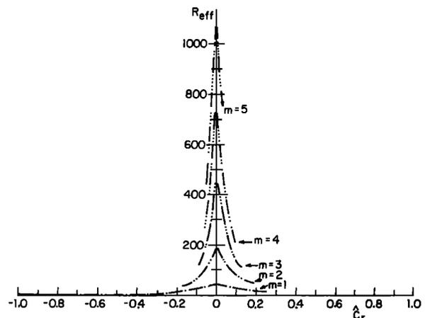
Fig. 8. Effective overreflection coefficient versus  $\hat{c}_r$  for the most unstable gravity waves as given in Figure 6. See Figure 4 for curve-labeling convention.
