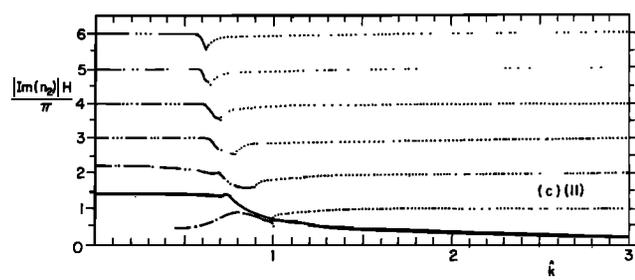
Fig. 5. Same as Figure 4 but for  $\hat{H} = 7.14$ . Now the most unstable gravity wave mode is  $m = 2$  (double-dot-dashed line).
