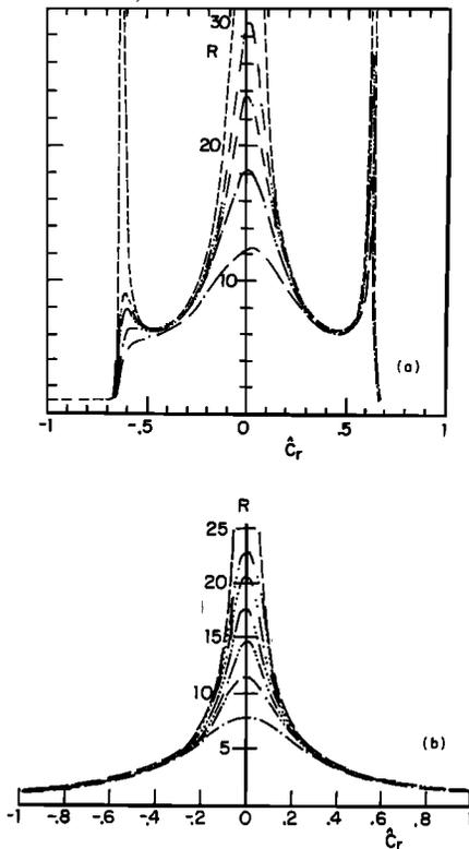
Fig. 7. Overreflection coefficient versus  $\hat{c}_r$  (dashed line) for (a)  $k = 0.6$  and (b)  $k = 0.48$ . Also shown are the effective overreflection coefficients based on growth rates for various mode numbers (see section 5 for details). See Figure 4 for curve-labeling convention for gravity waves.
