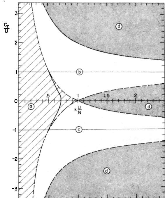
Fig. 2. Graph of  $c_r$  versus  $k$  for neutral radiating waves in unbounded fluid. Also shown are the various regions in  $k, c_r$  space discussed in section 2.
